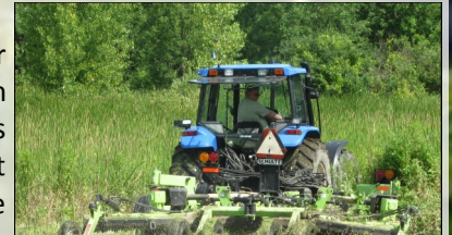
Bat Wing Deck can cut 15 feet in one pass
