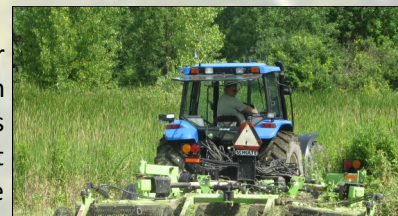
Bat Wing Deck can cut 15 feet in one pass
