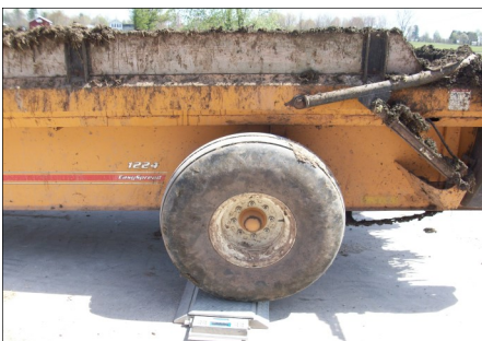
Calibrating a manure spreader for a CNMP involves weighing the spreader when it's full and when it's empty in order to determine the application rate
